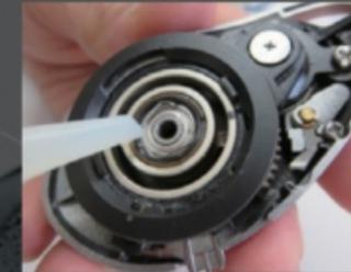
For other multiplier reels, apply a thin film of Maintenance Grease 104.
