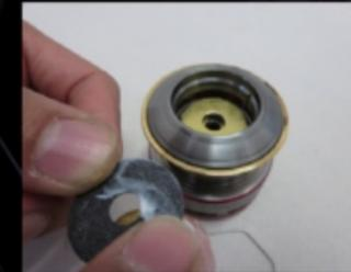
Apply drag washer grease to the drag washer.
