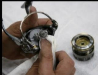
Wipe off the dirt from the upper area of the rotor.
