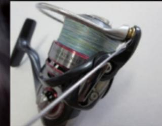
Apply spray grease to the line roller. This is unnecessary for MAGSEALED (Magnet Oil Shield) spinning reels.
