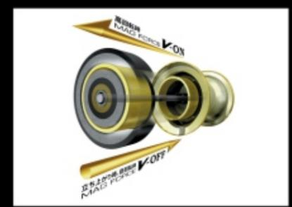
An advanced brake system that combines magnet brake system with centrifugal force system that, only applying brakes when the first half of the spool is cast. As it approaches maximum speed, the INDUCTOR ROTOR held by centrifugal brackets glides between the magnets to apply brakes, and retracts from the magnets as the spool begins to slow, so the spool keeps spinning longer.
