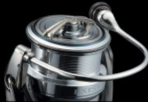
The smooth, protrusion-free design of the Airbail® allows line to slide easily down the bail onto the line roller as the reel is turned, reducing the problems of snagging or tangling. Because it features a hollow tubular design, maximum rigidity and strength is achieved with minimum weight.
