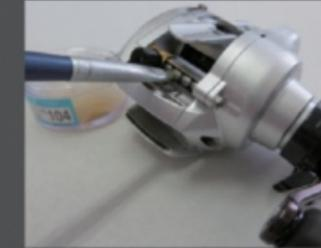
Apply Maintenance Grease 104 to the worm shaft.
