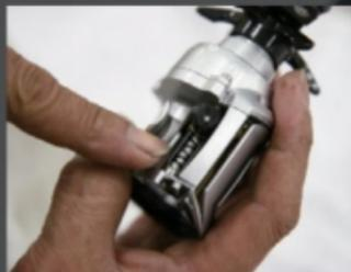
Check that no cloth fibers and lint are left on the worm and inside the frame during wiping, as these may cause a rotation failure.
