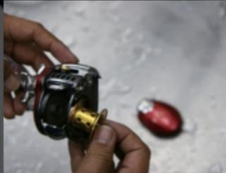
Tighten the drag all the way and wash away the dirt. For tough dirt, rub with a soft sponge soaked in a neutral detergent.
