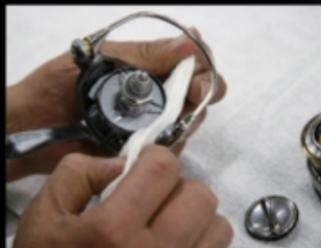
Wipe off the dirt from the side area of the rotor, which also can collect dirt.
