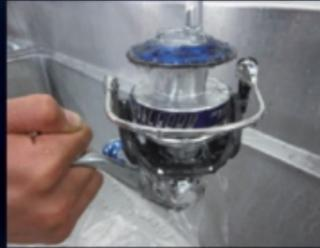
Apply running water from above to wash the reel. Do not rotate the handle.
