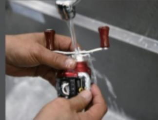
Wash the reel by rotating the handle. Rotate also the reel body while washing. Wash each face in running water for about 10 seconds.
