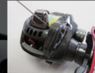
Apply spray grease to the joint of the smack lever
