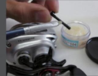
Apply Maintenance Grease 104 to the pinion shaft.
