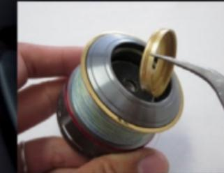
Reassemble the drag to complete the procedure. You can send the reel to us if there is any concern.
