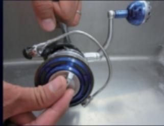
Tighten the drag adjustment knob while taking care not to cause water invasion into the drag.
